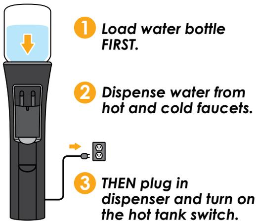
**⚠ WARNING: Dispense water through the hot and cold spigots before plugging in and turning on the hot tank heater switch. Failure to follow proper installation instructions may cause damage to water dispenser.**
