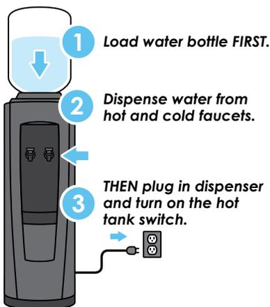
**⚠ WARNING: Dispense water through the hot and cold spigots before plugging in and turning on the hot tank heater switch. Failure to follow proper installation instructions may cause damage to water dispenser.**
